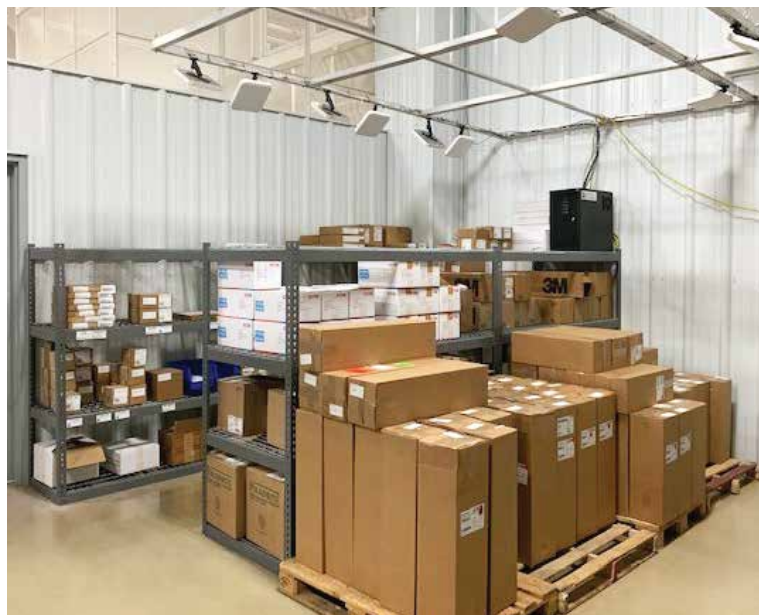
One of APC's SupplySentry installations: Two rows of shelves with an additional area for larger items. RFID readers hang above to monitor the whole area.
